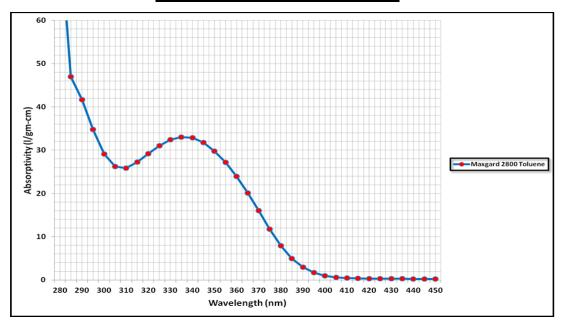
**MAXGARD 2800** is an effective light stabilizer for protecting plastics and coatings from the damaging UV radiation which is a component of natural sunlight. It is very compatible with several polymer materials and is very useful as a UV screen in these products.
